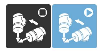
When is active align the axis Z of the current tool perpendicular to the plane X-Y of cobot base (with the Z direction entering the plane).
