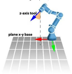
In this way we can obtain the cobot with a **exactly perpendicular orientation** to the working plane, which is impossible to obtain only with *Freedrive Mode* button.
