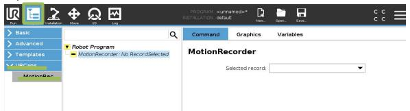
The block *MotionRecorder* has a drop-down menu with the list of recorded paths.
