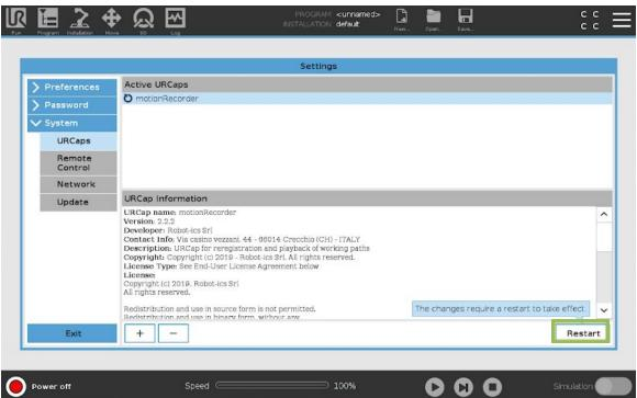
When the robot will be restarted Motion Recorder Software will be ready to be used. Following this procedure it is possible to install the software, but by default the version is limited, to unlock all the features of the **Motion Recorder Software** simply insert the dongle on a USB port of the cobot.
