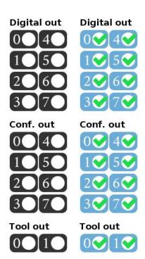
This buttons give the possibility to activate/deactivate a digital output without changing the window. The **Motion Recorder Software** in addition to the motion, will records the change of status of the digital outputs.
