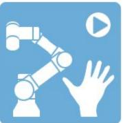
The *Freedrive Mode* button will active the freedrive mode of cobot. Pressing this button will be possible to move manually the cobot. In this status the cobot is in equilibrium, but if we apply any external pressure the robot will move in the force direction.
